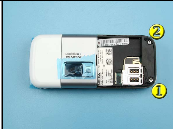
4. Undo the Torx Plus size 6 screws in the order shown. For assembly, use the reverse order and a torque of 15 Ncm.
