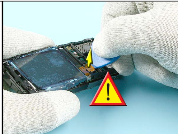
20. Now, also open the flex connector of the LCD MODULE.
