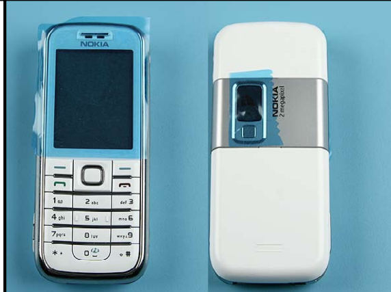
2. Protect the window with a protective film.
