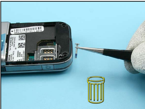
5. Discard the screws and use always new ones because of the locking compound.
