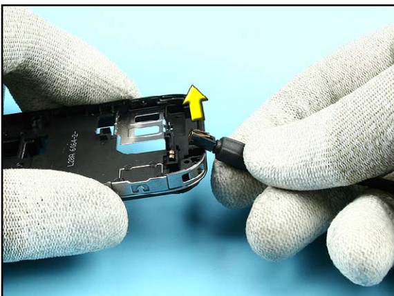
29. Remove the DC-JACK with a DC-plug.
