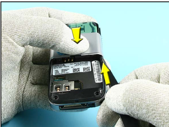
15. To release the CAMERA BEZEL, stick the closed tweezers between the CAMERA BEZEL and the D-COVER.
