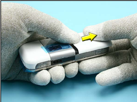
3. Open the BATTERY COVER and ensure that now battery is inserted.
